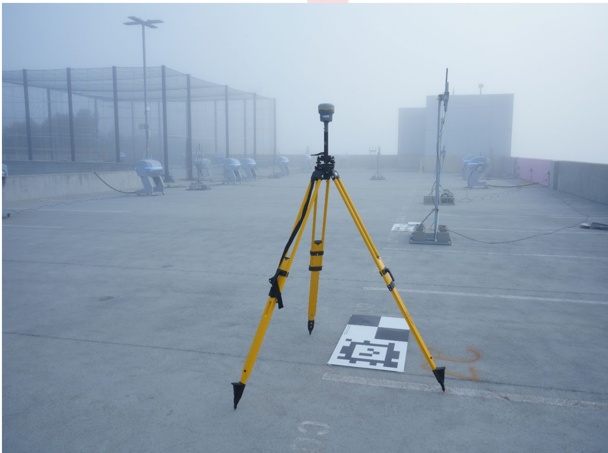
Trimble R12i observing the location of a static point
