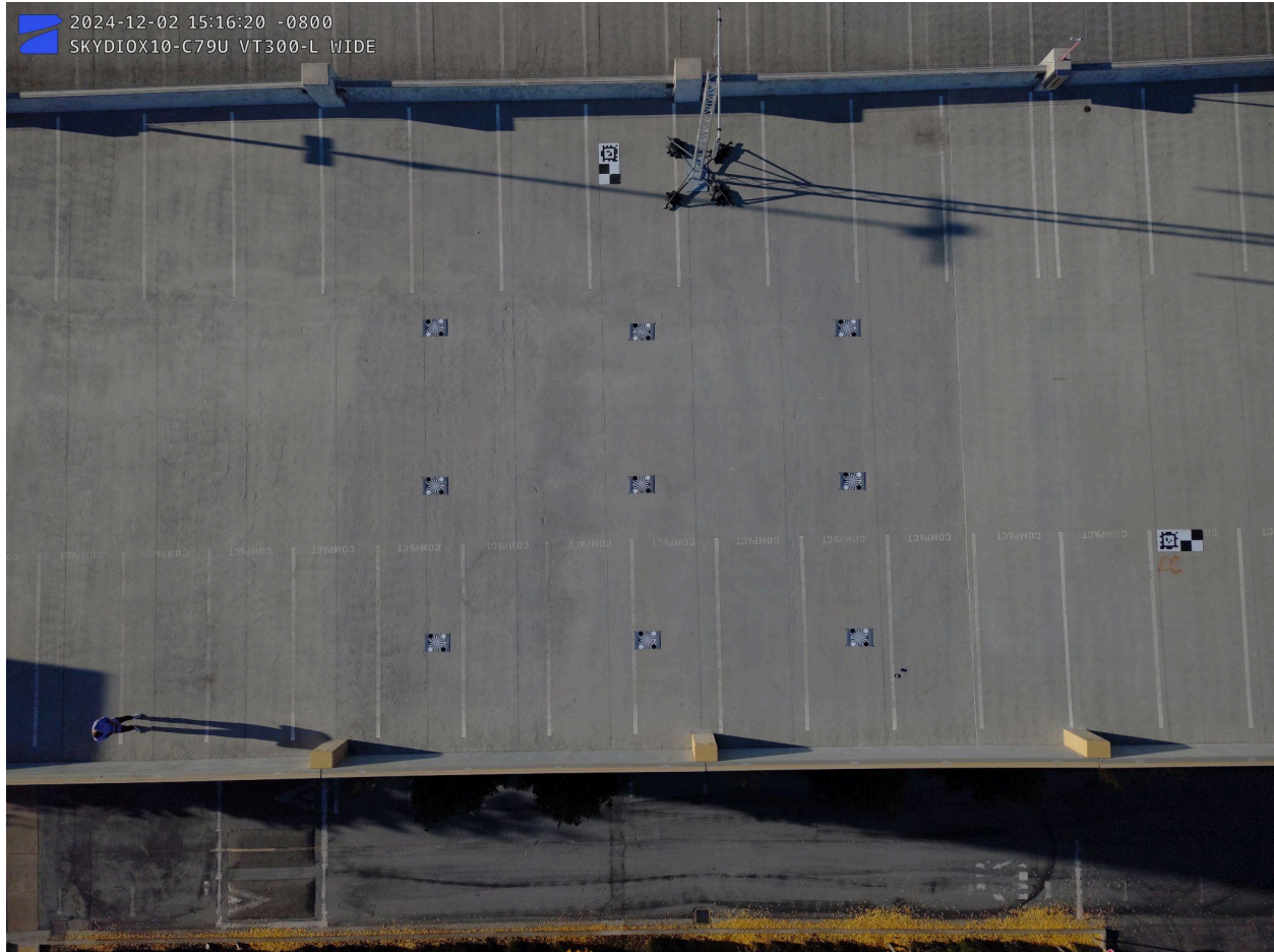
Distribution of the nine Siemens star targets on the ground
